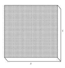
Nail four 2" x 4"x 3' boa together to form a 3'x (1meter) square. Staple gun fine mesh s the bottom.
